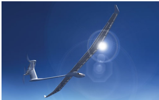
Solar Impulse has a 260-foot wingspan lined with solar panels.
