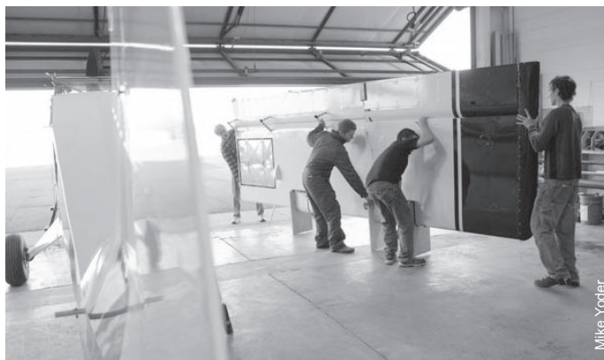
The GUT Works crew removed the second wing of the Husky in preparation for shipping it to Kenya. Handling the wing from left are GUT-Works manager Ron Renz, mechanic Phillip Pützer, base mechanic for LifeStar Paul Isabell, and Jonah Seibel.
