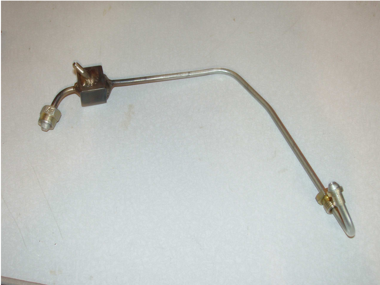
Photo 1. Modified Injector line. This modification allowed testing of a piezo electric element by direct exposure to the high pressure of an injection event. It also allowed direct measurement of the pressures in the injection event.
