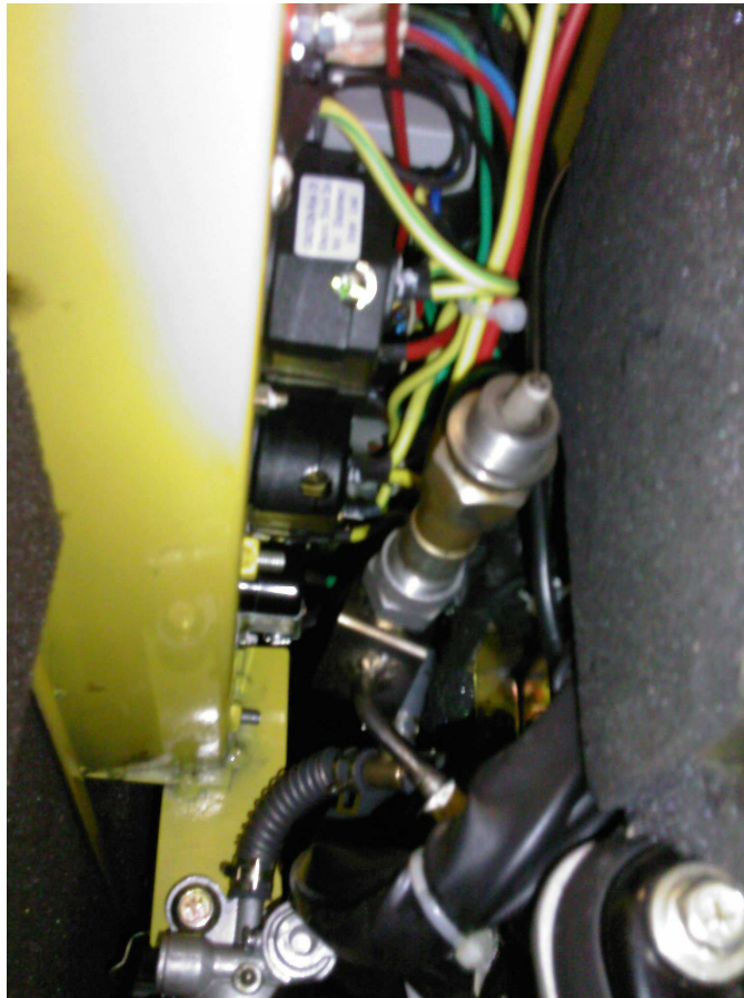
Photo 3. Piezo ignitor/plug assembly installed on the modified injector line for operational testing.
