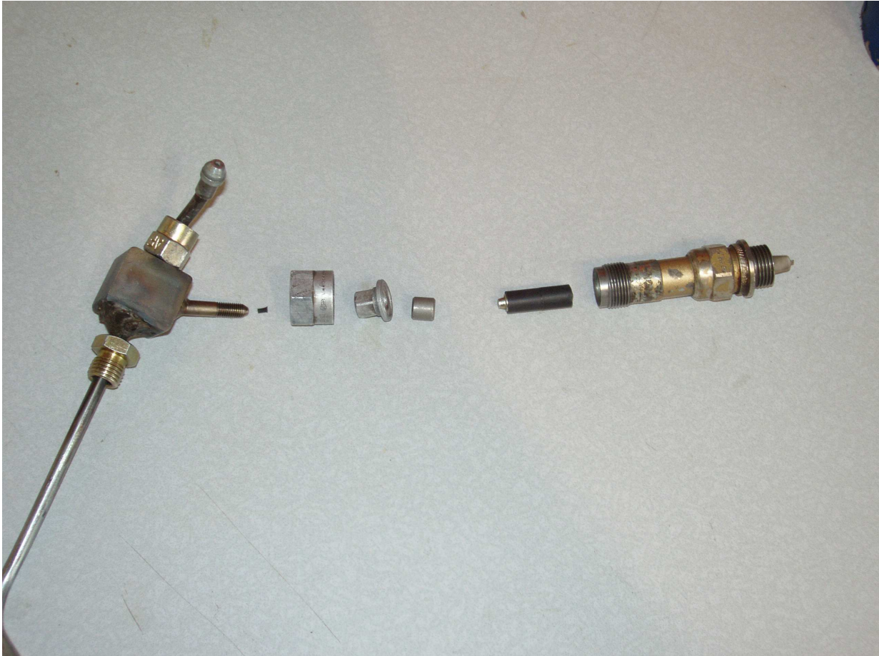
Photo 2. Exploded view of the piezo element test assembly. The ignition capsule is the black cylinder with the silver tip. This fit directly into the modified spark plug barrel insulator for signal measurement.
